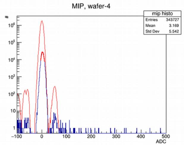
**COSMICS : threshold calculated with 5sigmas, find noisy with thresholds 0.05 and 0.01 (only 10 minutes)**
