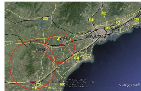
Figure 3.3: Illustration of the CEPC-SPPC ring sited in Qinghuangdao. The small circle is 50 km, and the big one 100 km. Which one will be chosen depends on the funding scenario.
