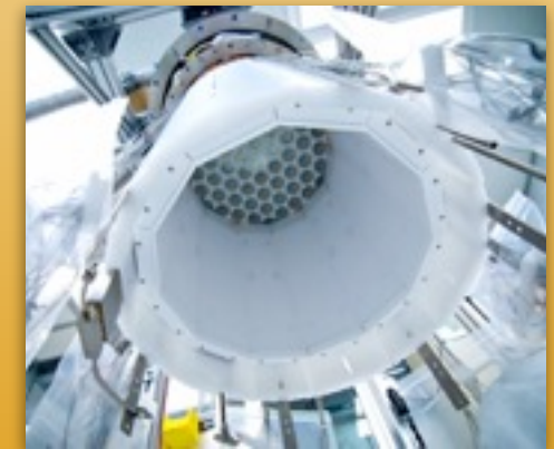
Active region defined by PTFE reflectors (high reflectivity >97%) - high light collection
