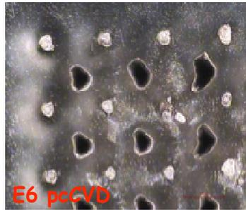
1064 nm YAG ns laser ablation of pcCVD
