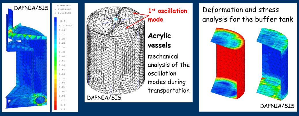
Acrylic double vessel max stress: 1.2 MPa
