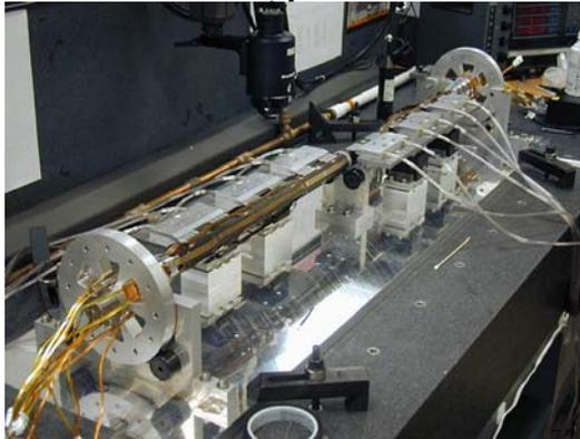
Example 1: Liverpool designed & manufactured the supports for the L00 CDF layer (i.e. low mass cylindrical rigid structure of Radius = 1.5 cm and incorporating strips & cooling channels
