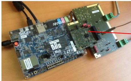
SAMPA ASIC bonded on PCB
