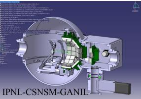
The mechanical design foresees the use of 54 self produced NEDA detectors at forward angles and 14 NWALL detectors at around 90 degrees coupled to DIAMANT, using the NUMEXO2 FEBEE
