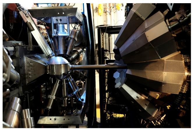
35 detectors on-line : Single efficiency measured at 3.4(1)% in nominal position at 1.408 MeV (GEANT4 = 3.6%)
