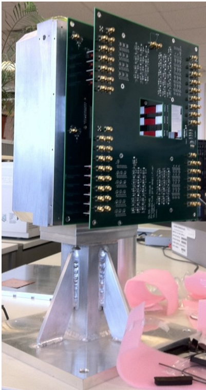
Cryostat and preamp board
