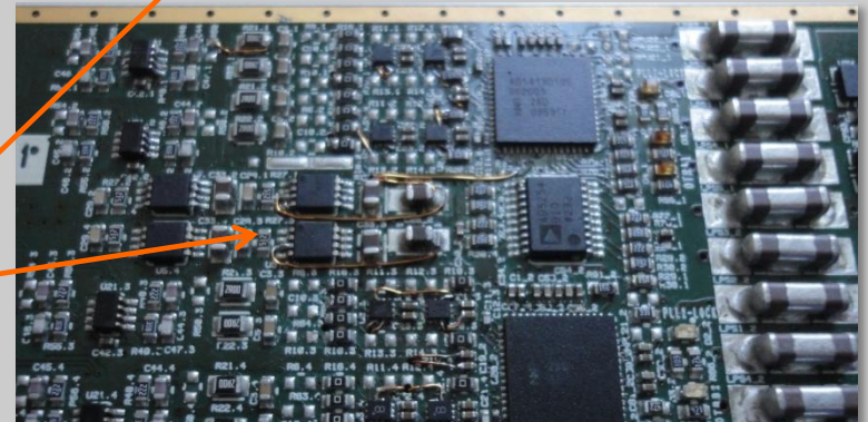
Card 3 core – Missing vias shorted by “flying” wires
