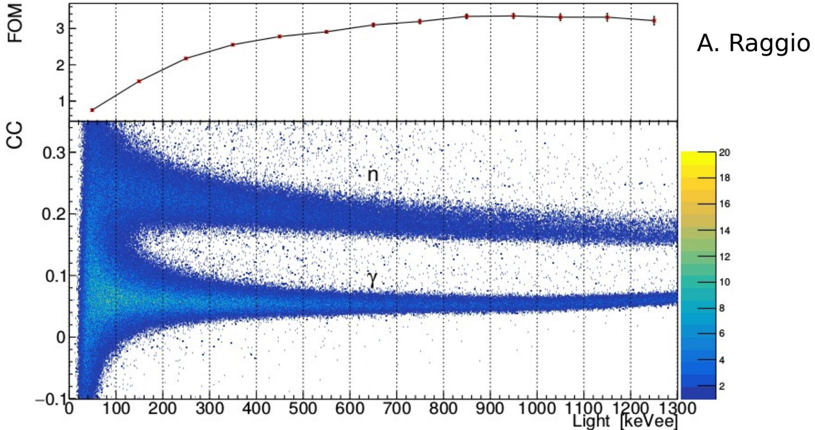
Figure 3.15: 2-D density plot of CC vs Light. The top line shows the FOM value for each energy gate.
