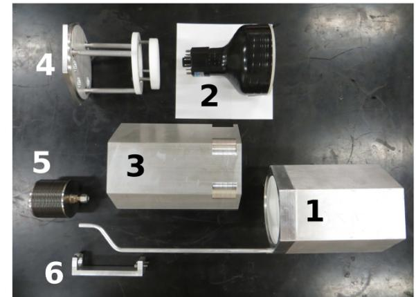
Fig. 1. Elements used for the construction of the NEDA detector: detector cell, with extension pipe (1); PMT (2); PMT housing (3); PMT pusher (4); the bellow (5) and the support for the bellow (6).
