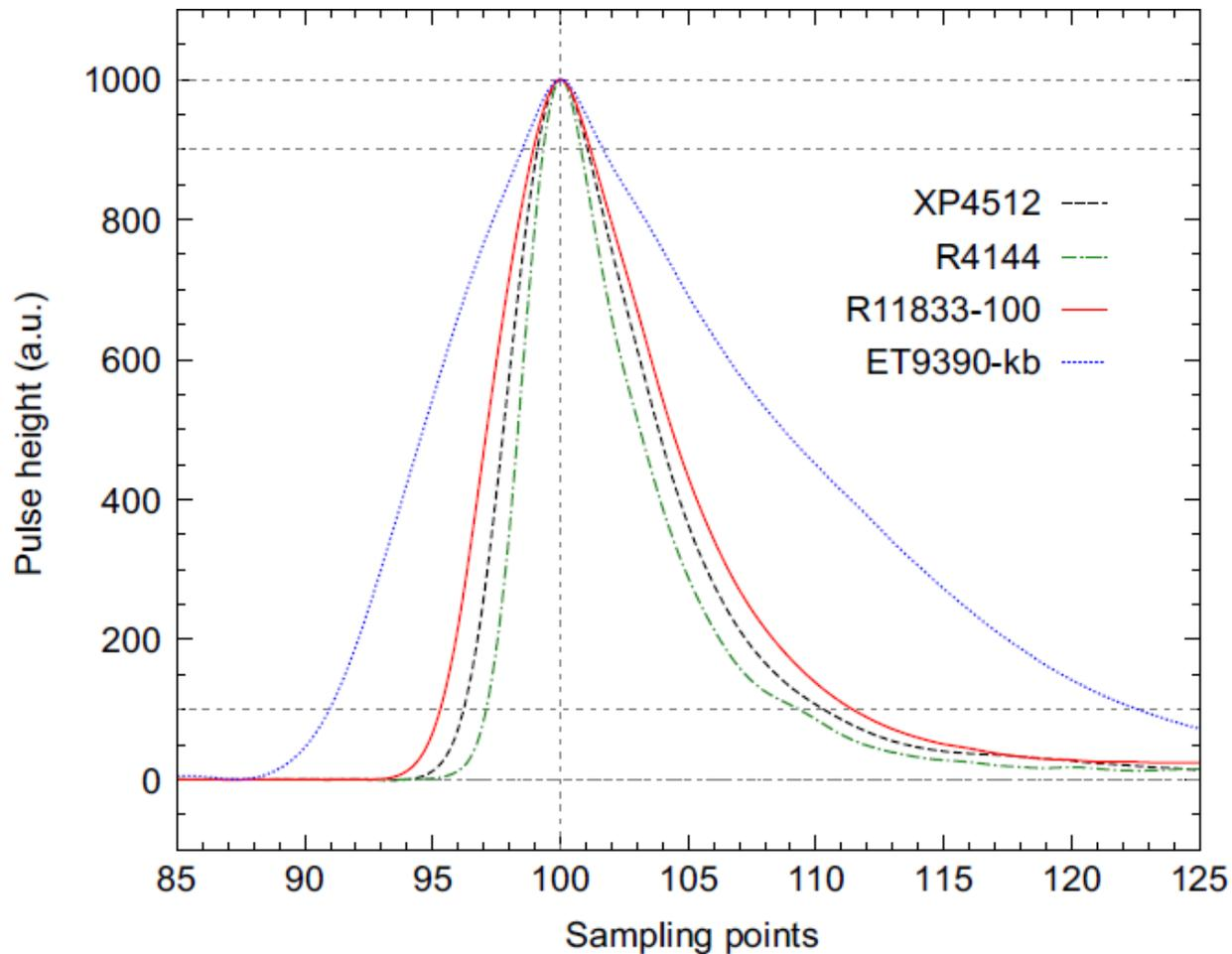
**Fig. 2.** Digitized waveforms averaged over  $10^5$  events for the four 5 in. PMTs coupled to a cylindrical 5 in. by 5 in. BC501A. The sampling frequency of the digitizer was 500 MS/s. The waveforms were normalized to a pulse height of 1000 and time aligned at the maximum of the signal. Dashed lines are drawn at 10%, 90%, at the maximum and at the baseline of the waveform to guide the eye.
