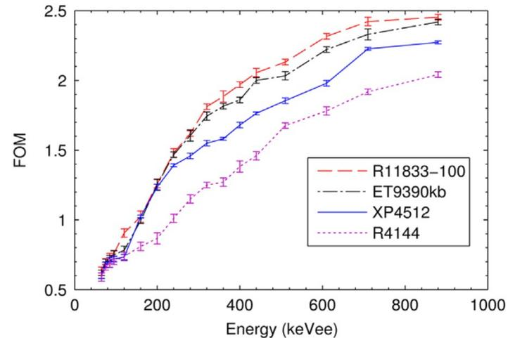
**Fig. 10.** FOM values of the IRT method for PMT ET9390kb, R11833-100, XP4512, and R4144 as a function of energy window (the widths of the windows are 10, 40, and 100 keVee in energy regions of 50–100, 100–500, and 500–1000 keVee, respectively).
