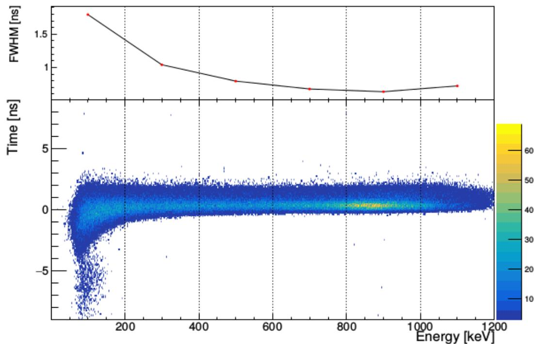
Figure 3.9: Digital timing distribution as a function of energy. The top line shows the FWHM for each corresponding energy gate.
