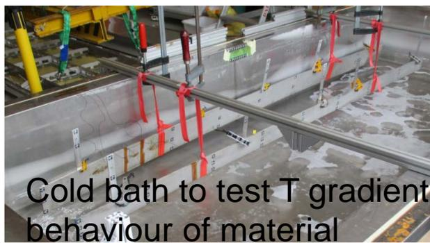
Cold bath to test T gradient behaviour of material
