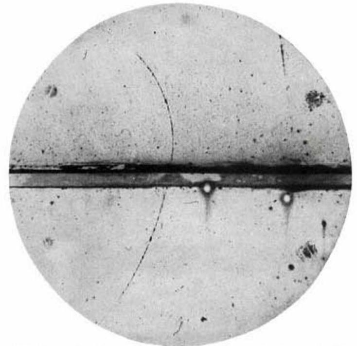
Fig. 1. A 65 million volt positron ( $H_p = 2.1 \times 10^6$  gauss-cm) passing through a 6 mm lead plate and emerging as a 23 million volt positron ( $H_p = 1.5 \times 10^6$  gauss-cm). The length of this latter path is at least ten times greater than the possible length of a proton path of this curvature.
