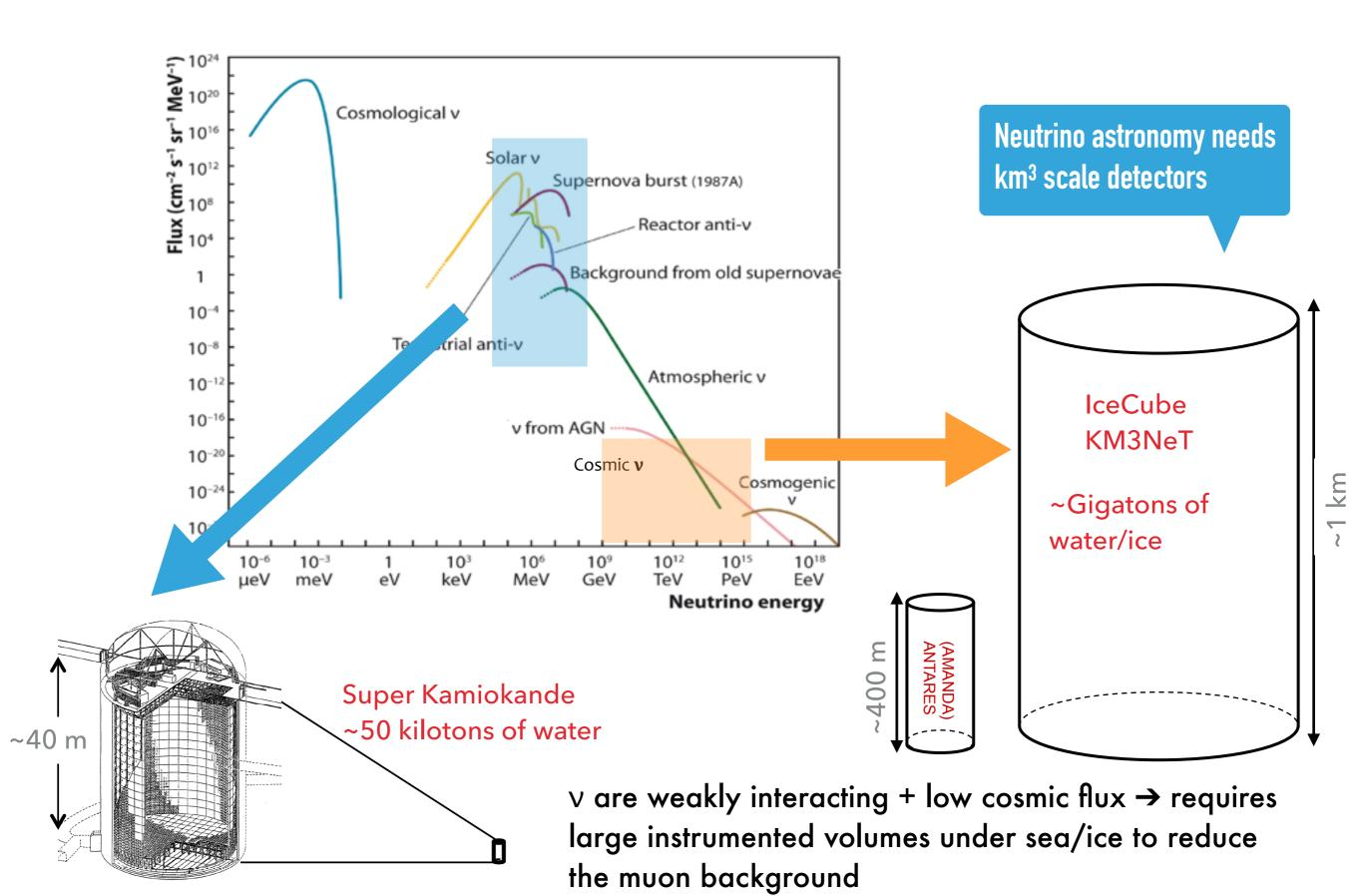
Different ways to detect HE  $\nu.$  One way particularly useful in astronomy: observation of muons produced in CC interaction of  $\nu_\mu$
