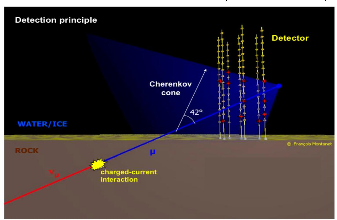
Different ways to detect HE  $\nu.$  One way particularly useful in astronomy: observation of muons produced in CC interaction of  $\nu_{\mu}$
