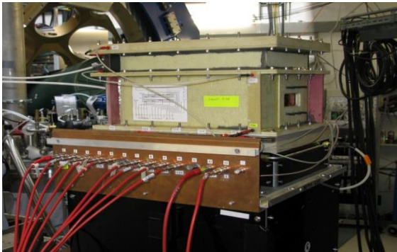
O-TPC: discovered \beta -delayed 3p-emission of ^{31}\text{Ar}
