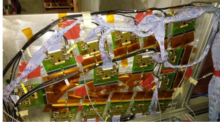
Full size GEM detectors tested with free-streaming read-out electronics at the CERN-SPS Nov.-Dec. 2016
