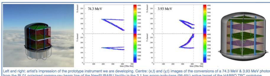
Left and right: artist's impression of the prototype instrument we are developing. Centre: (x,t) and (y,t) images of the conversions of a 74.3 MeV & 3.93 MeV photon from the BL01 polarised gamma-ray beam line of the NewSUBARU facility in the 2.1 bar argon-isobutane (95-5%) active target of the HARPO TPC prototype.
