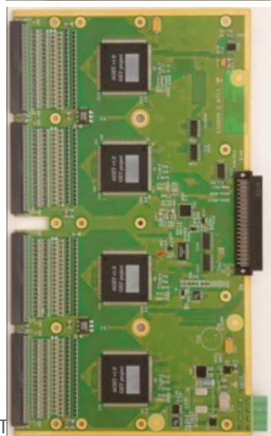
MINOS FEC: 4 AGET chips (pin-compatible with AFTER)
