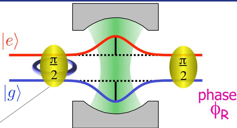
1. Trigger of the atom clock: resonant  $\pi/2$  pulse
