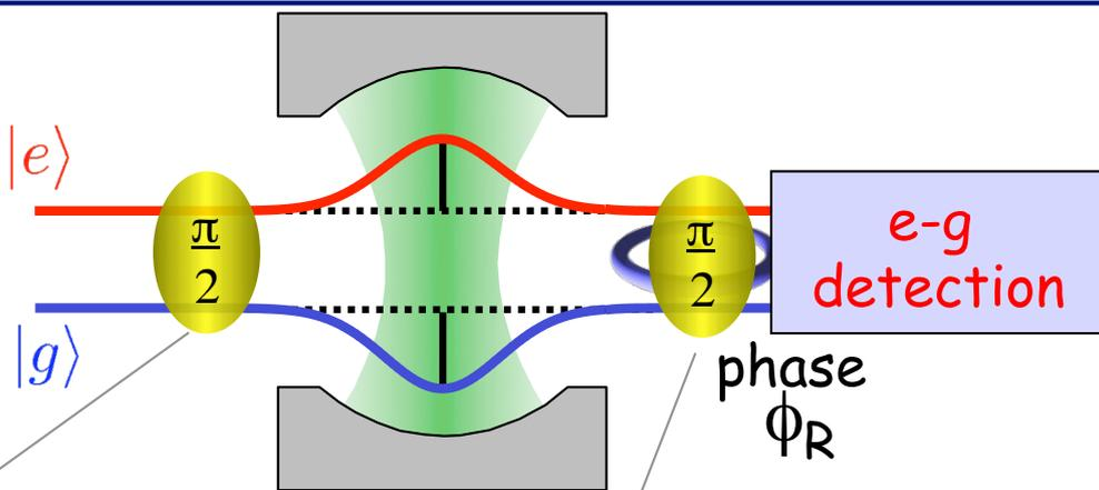
1. Trigger of the atom clock: resonant  $\pi/2$  pulse
