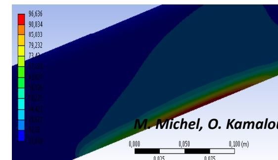
➤ Cooling :  $T^\circ < 100^\circ \text{C}$  for 1 kW losses
