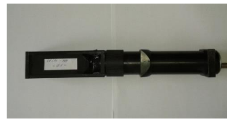
Plastic scintillator (4x4x12 cm 3 ) couplet to PMT
