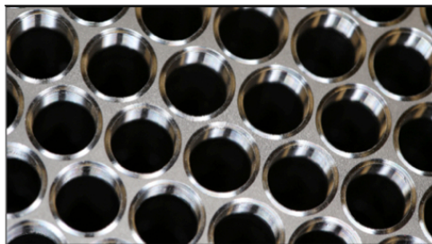
Petal (1/10 focal plane) and 1st fiber positioner
