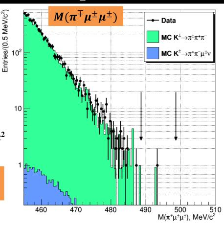
Events in Signal Region observed after  $K^{\pm} \to \pi^{\mp} \mu^{\pm} \mu^{\pm}$  selection:  $N_{obs} = 1$  Expected background (from MC):  $N_{exp} = 1.163 \pm 0.867_{\text{stat}} \pm 0.021_{\text{ext}} \pm 0.116_{\text{syst}}$  From Rolke-Lopez statistical method:  $BR(K^{\pm} \to \pi^{\mp} \mu^{\pm} \mu^{\pm}) < 8.6 \times 10^{-11}$  @ 90% CL
