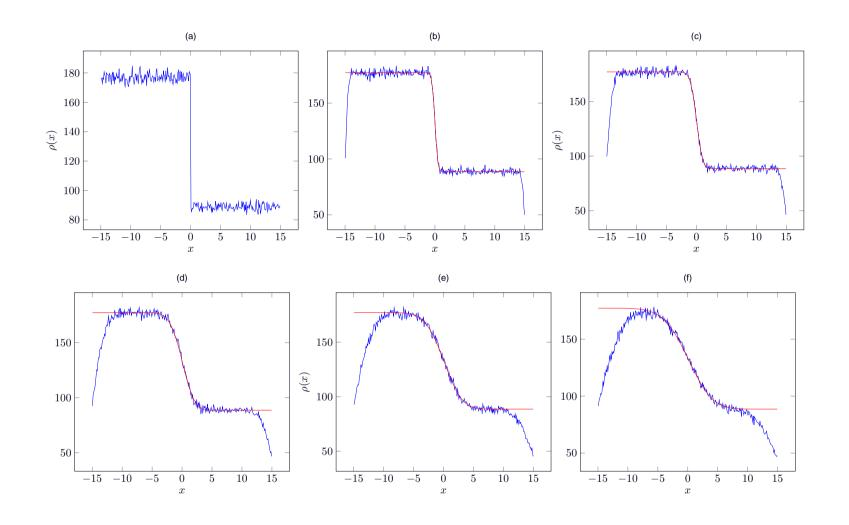
Figure 1: Hard rod density at times (a) t=0, (b) t=0.5, (c) t=1, (d) t=2, (e) t=3, (f) t=4, rod length a=0.001. Simulation data in blue, exact solution in red. [BD, Spohn 2017]
