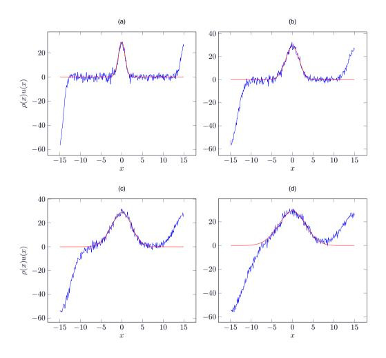
Figure 2: Current at times (a) t=1, (b) t=2, (c) t=3, (d) t=4. , rod length a=0.001. Simulation data in blue, exact solution in red. [BD, Spohn 2017]
