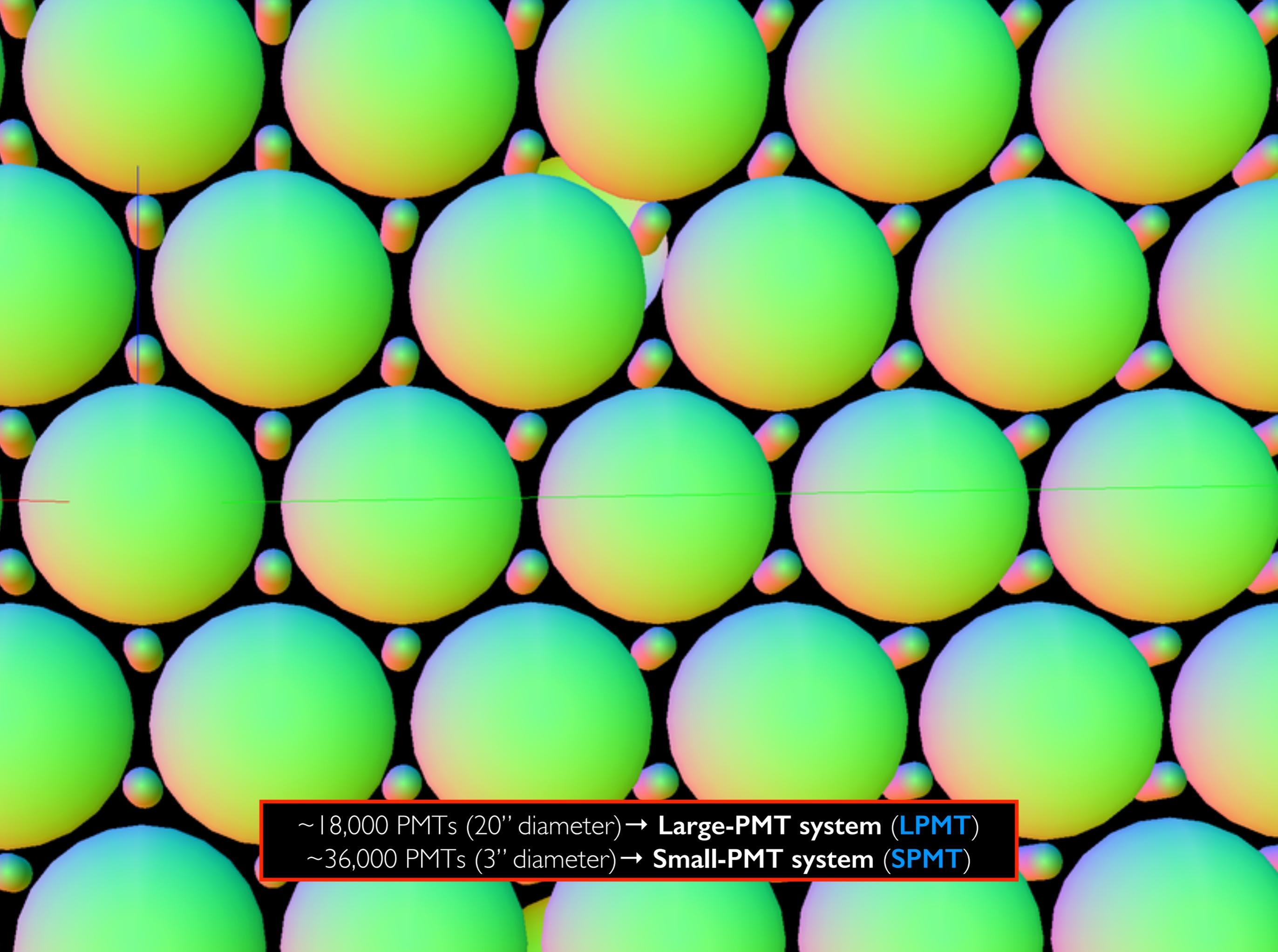
~18,000 PMTs (20" diameter) → **Large-PMT system (LPMT)**
