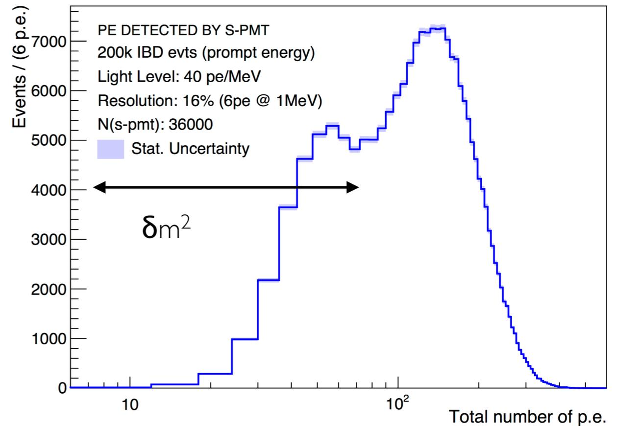
SPMT system alone can measure **solar parameters**  $\sin^2(2\theta_{12})$  and  $\Delta m^2_{12}$
