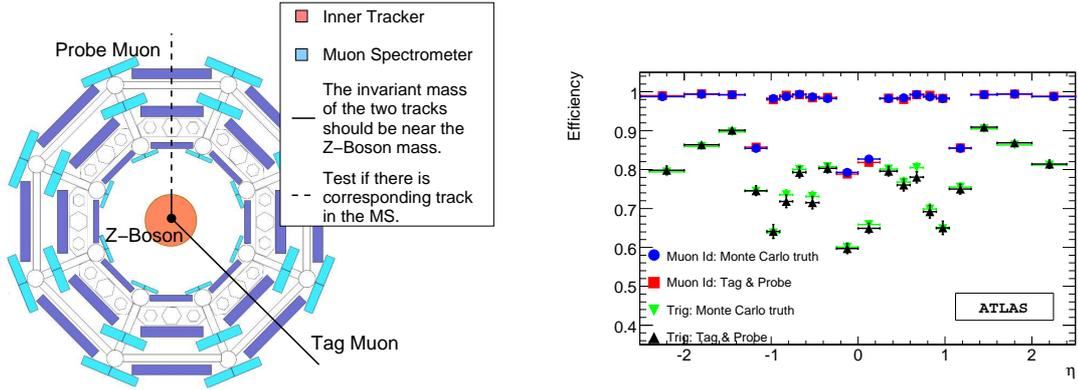
Figure 3: Left: Schematic illustration of the tag and probe method. Right: Muon detection efficiency vs.  $\eta$ , as measured from the tag-and-probe method and compared to the truth, for  $50 \text{ pb}^{-1}$ . The 20 GeV single muon trigger efficiency and the combined muon reconstruction efficiency are represented.
