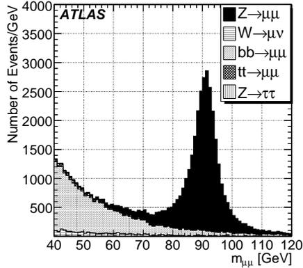
Figure 2: Di-muon invariant mass distribution in the  $Z \rightarrow \mu^+\mu^-$  channel, for signal and background, for  $50 \text{ pb}^{-1}$ , after all cuts, except the isolation and  $M_{\mu\mu}$  cuts.
