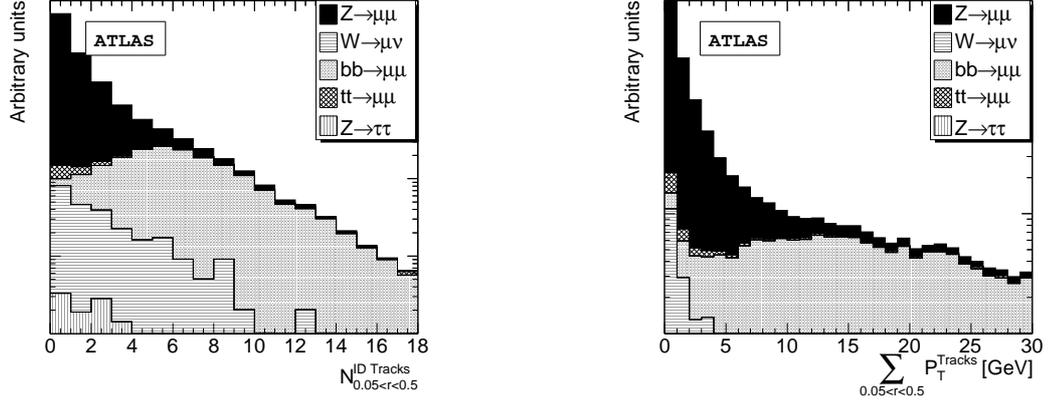
Figure 1: Isolation variables for signal and backgrounds after all selection cuts. Left: Distribution of the track multiplicity within  $\Delta R = 0.5$  around the muon. Right: total transverse momentum of tracks within the same cone around the selected muon.
