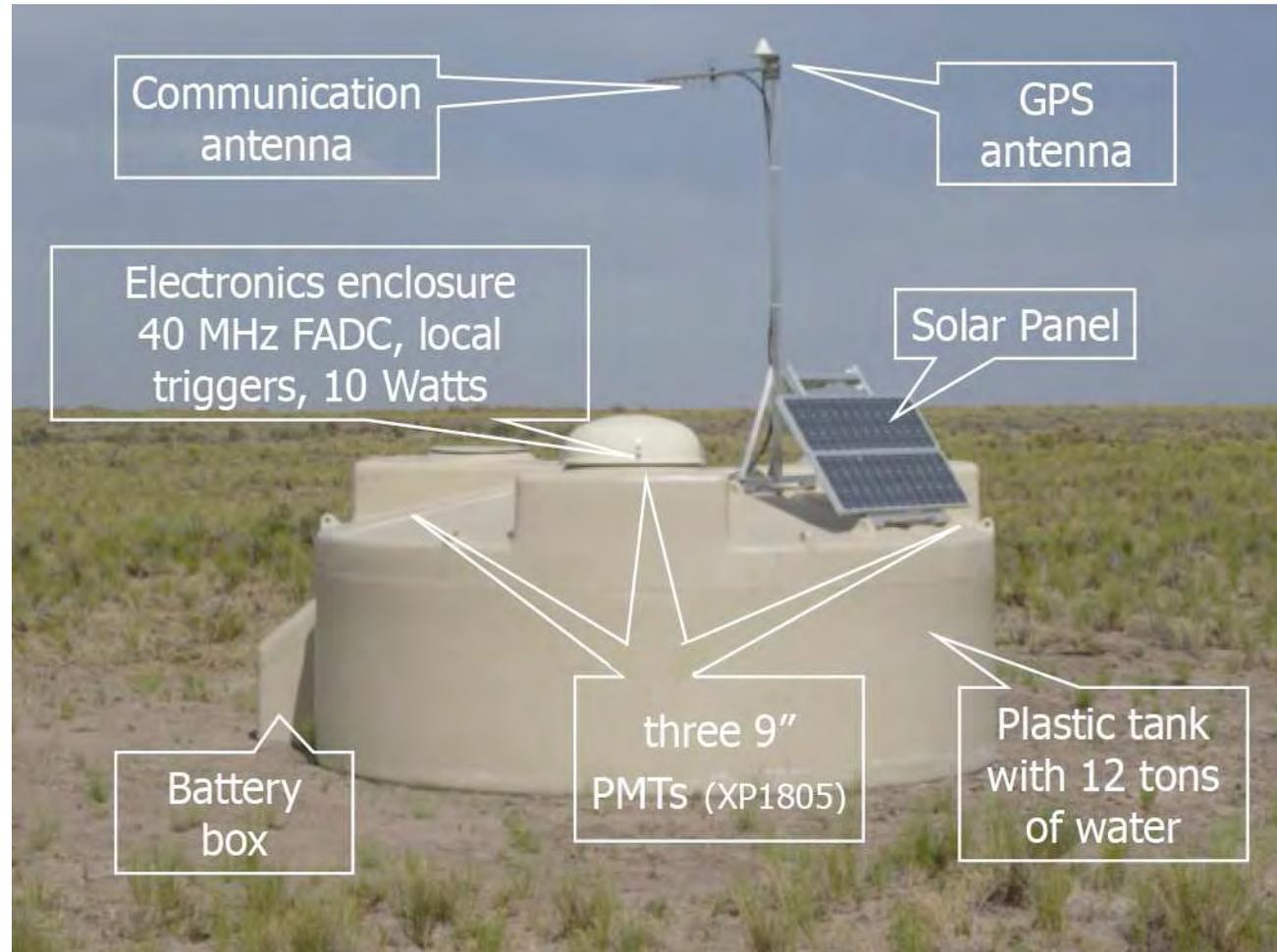
**DAQ : 40 MHz FADC sampling (10 bit resolution)**
