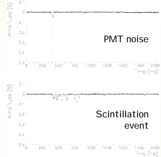
The different time characteristics of PMT noise (decay time of order of tens of ns) and of scintillation event (decay time about 240 ns) can be investigated building several variables
