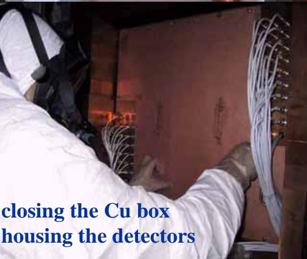
closing the Cu box housing the detectors
