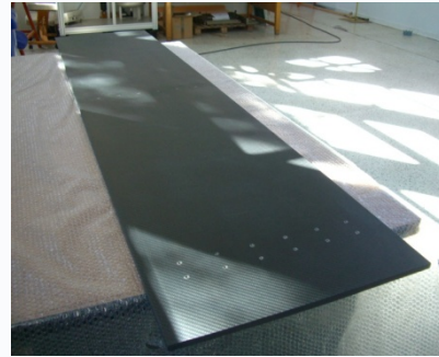
End-Cap thick composite plate 13mm+ inserts for double row rails
