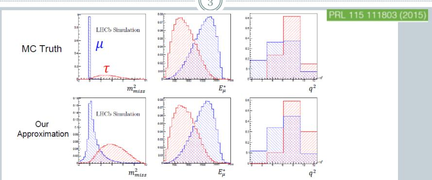
Using the known B flight direction, approximate the B momentum using  $y\beta_{z,vis}=y\beta_{z,B}$ :
