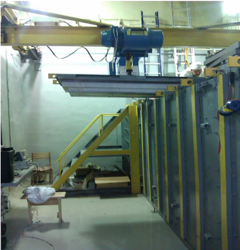
Passive shielding of 60 tons
