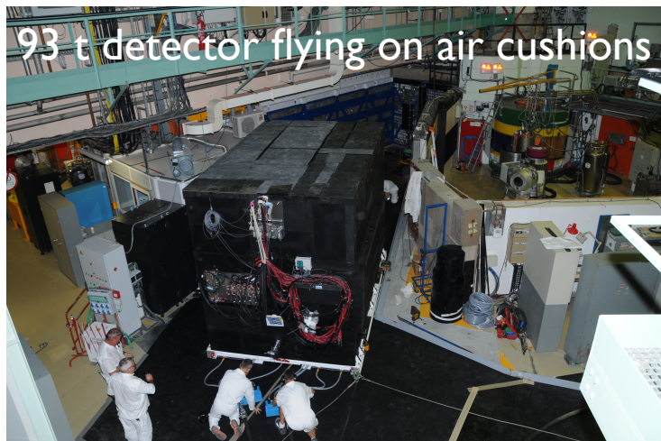
Insertion underneath the ILL water channel
