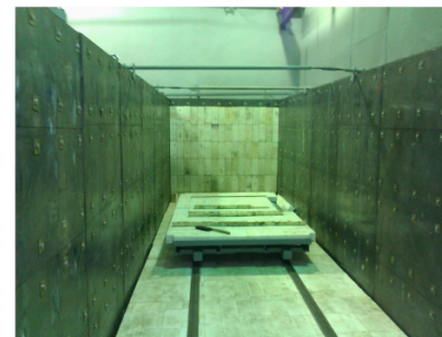
combined shielding for n and gamma-rays
