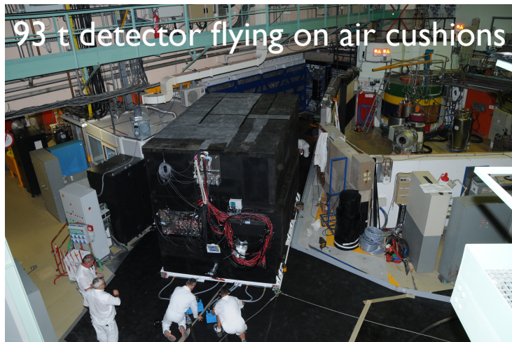
Insertion underneath the ILL water channel
