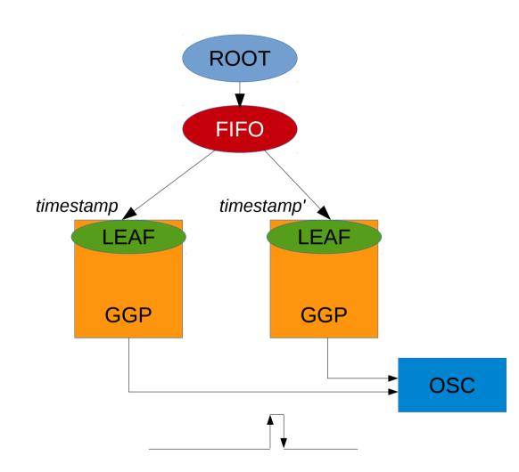
Monitoring the signal produced by the timestamp when generating the sync pattern using the sumbus interface
