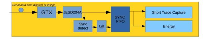
• The logics involved in the deserialization, link stablishment, synchronization, trace capture and energy fits the functionality of a CHANNEL
