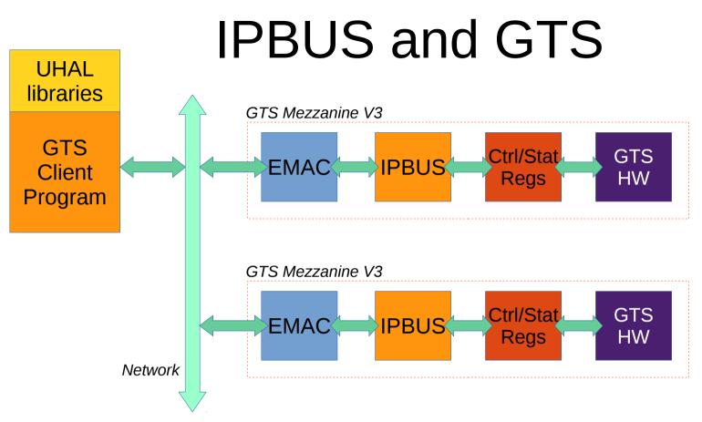
IPBUS solution proposed as an alternative to simplify the GTS control system.
