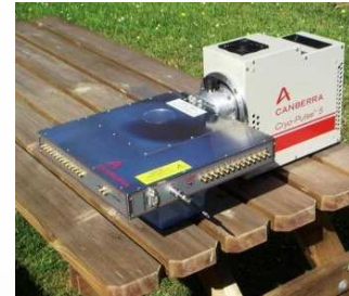
Single electrically-cooled DSSD for Compton imaging (Si(Li) or HPGe)
