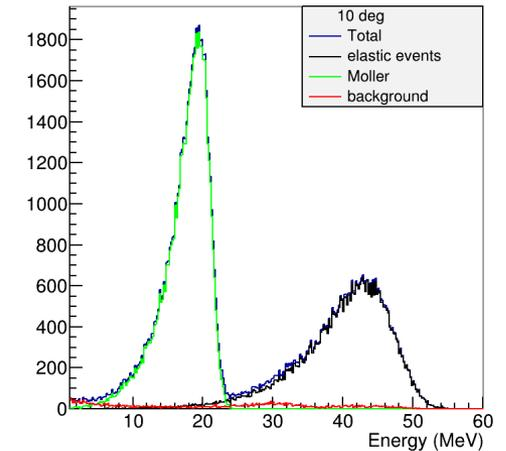
□ Absolute **normalization** from **simultaneous** measurement of **ep elastic** and **ee Møller** within the **same detector** using scattered electron kinematic separation.
