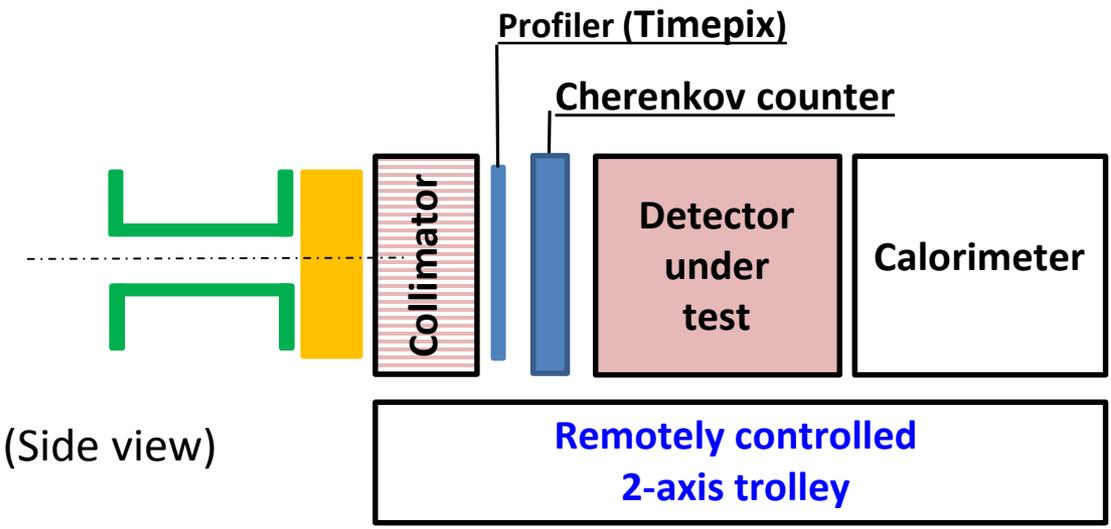
Timepix detector for precision spot measurement
