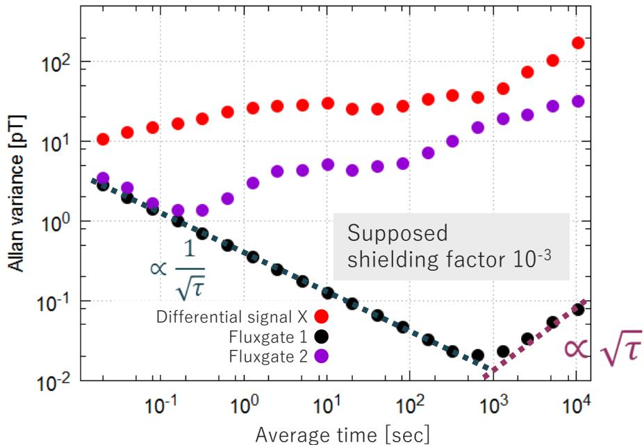
Magnetic field fluctuation is large on one side of the shield → Correction coil is needed
