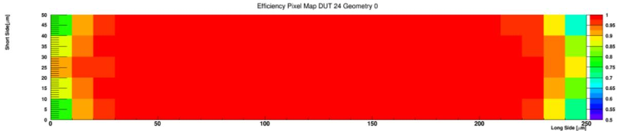
Lack of efficiency at the border due to punch through structure
