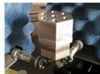
Feed+OMT array under test
