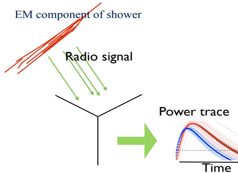
When developing in the atmosphere the electromagnetic cascade radiates in the microwave band. Each microwave antenna measures continuously the radiation of the cascade as a function of time. The interface electronic converts this signal to its power envelope and feed it to the tank front end electronics.
