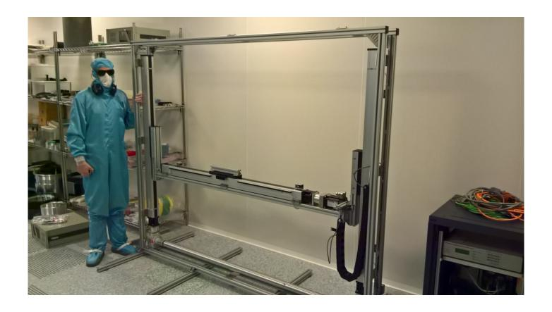
Installation of the optical bench (developped for the actual LSST filter) in the ISO3 cleanroom
