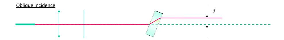
Beam displacement due to the refraction in the substrate
