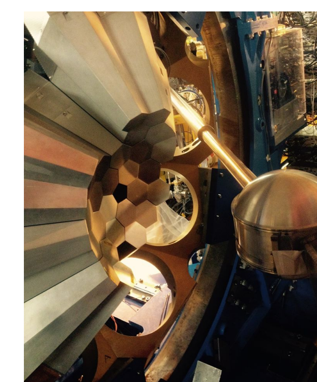
Fig. 8: Picture of the AGATA detectors
