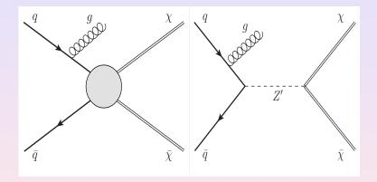
Jets + \$\vec{E}\_T\$ signal interpretation in terms of (a) contact interaction described by EFT operators and (b) a simplified model with s-channel Z' boson exchange
