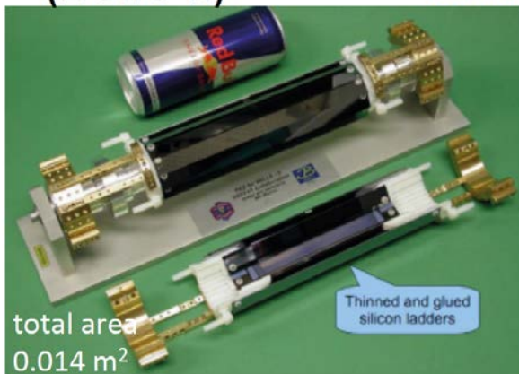
STAR Heavy Flavour Tracker (HFT) at RHIC - Installed 2013 [L. Greiner, FEE 2014]
