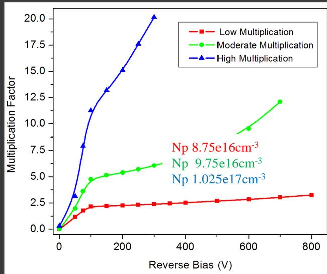
The reason for higher multiplication factor is that the localised electric field peaks up with increasing p-well concentration.
