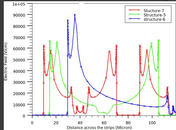
As the strip pitch increases, the electric field at the implant edge rises.
