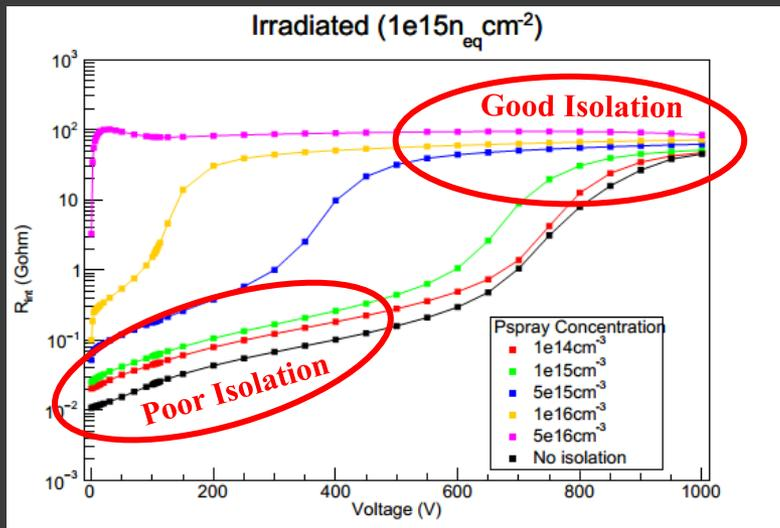
A higher concentration & a deeper pspray/pstop provides good isolation. But, this also leads to a rise in the electric field!
