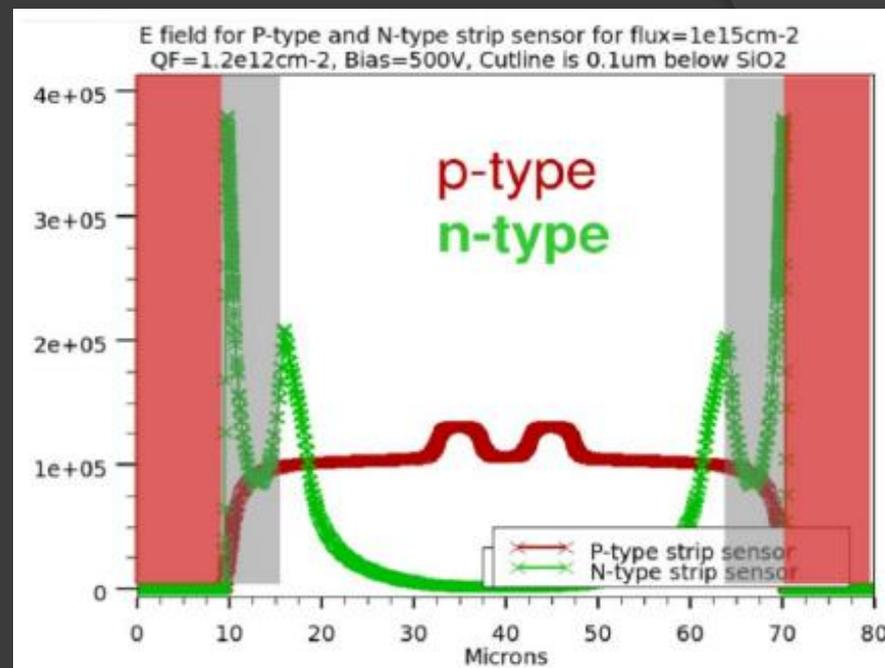
Increasing fluence  $\rightarrow$  More radiation damage  $\rightarrow$  Higher bulk & surface damage  $\rightarrow$  Qf grows  $\rightarrow$  E.Field @ implant edges shoots!
