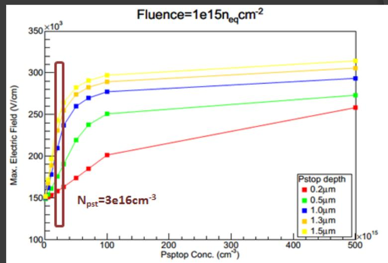
Therefore, an optimized concentration & depth of the isolation structure has to be chosen.
