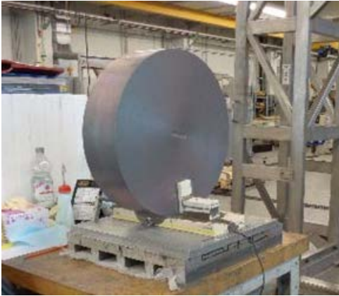
CBMM ingot. \varnothing=480 mm RRR>300
