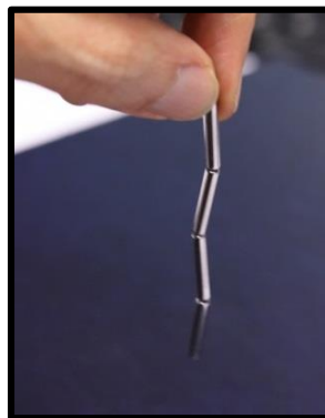
Bearing cage and needles magnetized
