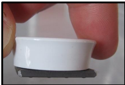
Bearing cage and needles magnetized
