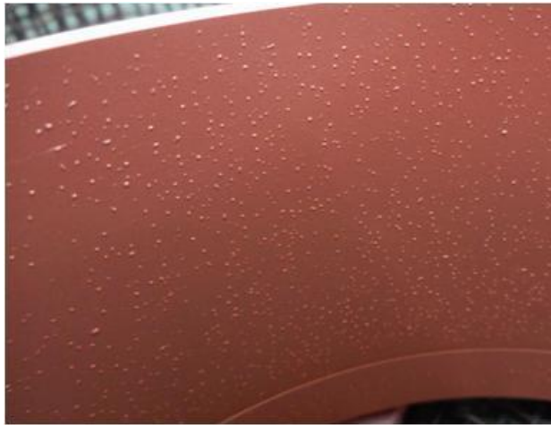
Many large blisters on the inner surface after heating
