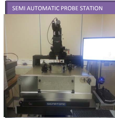
Measurement from -60 °C to 300 °C
