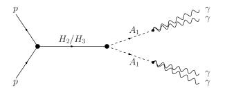
Viable if  $M_{A_1} \lesssim 800$  MeV; then the photons from  $A_1$  decays are sufficiently collimated such that they appear (mostly) as a single photon in the electromagnetic calorimeters (see below)
