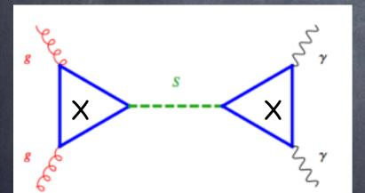
$$c_{sgg} = \frac{y_X v}{12\pi^2 m_X}, \qquad c_{s\gamma\gamma} = \frac{y_X Q_X^2 v}{2\pi^2 m_X}$$
